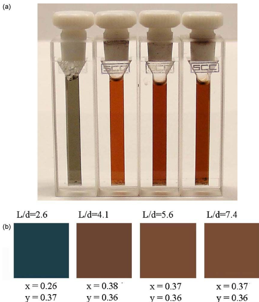
Fig. 7. (a) Photograph of 4 sols of colloidal gold prepared in water. Aspect ratios are 2.6, 4.1, 5.6 and 7.4 (from the left), respectively. (b) The simulated color of dispersion of gold nanorods of different aspect ratio [125].
