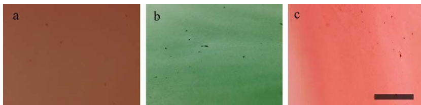
Fig. 14. Optical micrographs of drawn PVA-gold nanocomposites (4% w/w gold, draw ratio 4): (a) unpolarized, polarization direction, (b) parallel and (c) perpendicular to the drawing direction. Scale bar is 50\ \mu\text{m} [125].
